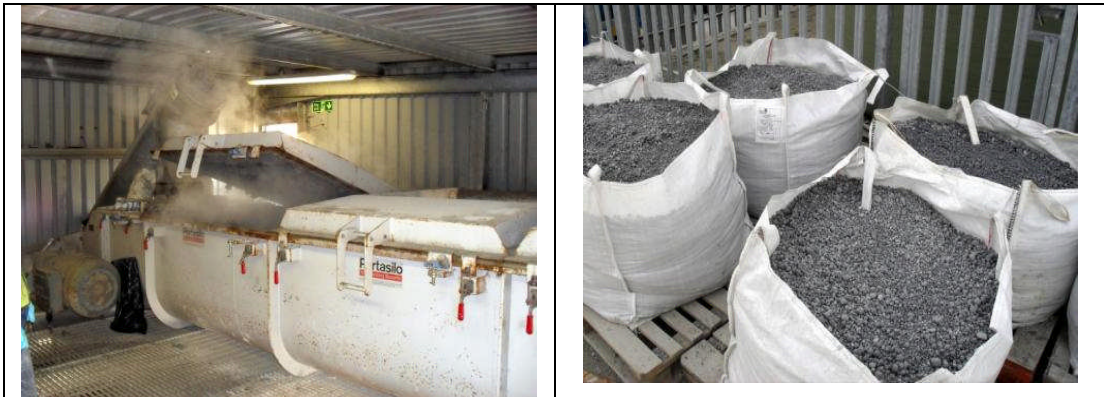
Figure 3. Pilot scale trial; pre-treatment mixer (left), tonne bags of carbonated aggregate (right)
